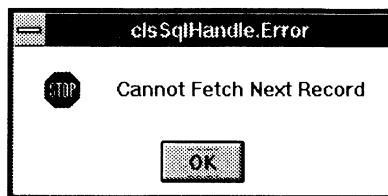
Figure 4.6 Message box to indicate the error message in case dfName was declared of data type Number instead of String.
